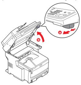
2. If a sheet is well advanced out of the top of the printer, simply grip it and pull gently to draw it fully out. If it does not remove easily, do not use excessive force. It can be removed from the rear later.
